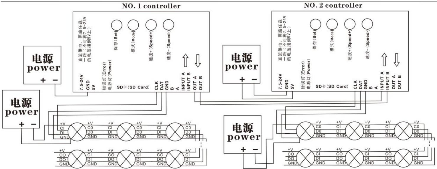
1. Multiple T-1000S controllers can be cascaded together and work synchronous.
